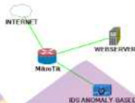
Gambar 4.1. Topologi jaringan IDS anomaly-based
