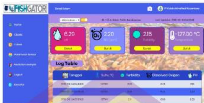
Gambar 6. Tampilan Dashboard Web Services Sistem Monitoring Kualitas Air Kolam
